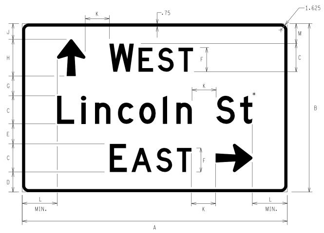
$\begin{array}{c} \text{D3-2} \quad \text{(1.6)} \\ \text{ADVANCE STREET NAME (WITH DOUBLE CARDINAL DIRECTIONS)} \\ \text{FOR DIRECTIONAL CROSSOVERS ONLY} \end{array}$
